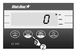
2. Pressing displays zero weight and flashing arrow on side of display points to NET.
